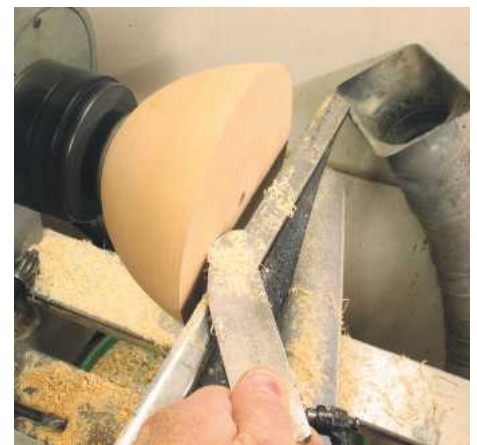
▲ Pic.5 If you need to scrape the inside of the bowl, then do it in stages. As you remove wood, the bowl can start to go out of shape, so scrape each section to a finish before following the next part
